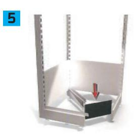
Fit the plinth skirting into position by slotting it between the front capping on the baselegs.
