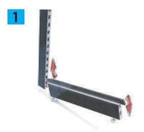
Locate the baseleg rear lug and block into the bottom "H" Slots of the upright as shown.
