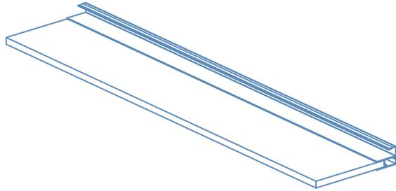
Step 1: Install the No. 4 wooden board into the slot of No. 3.
