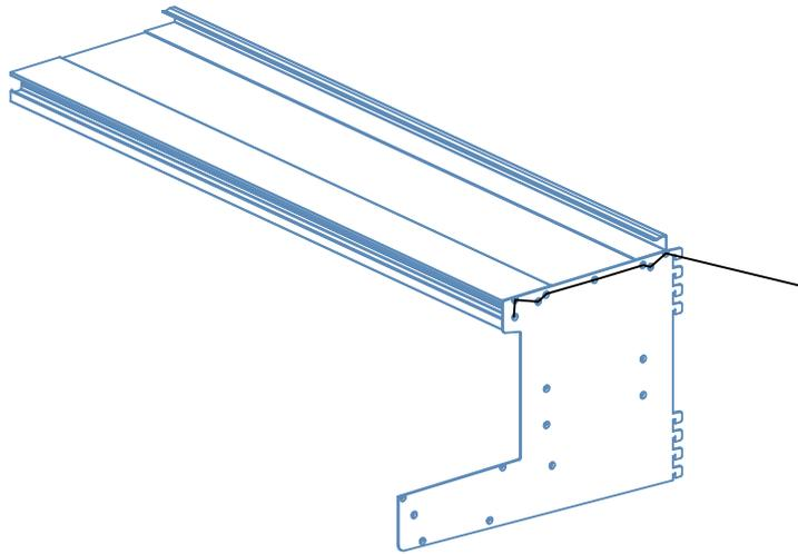
Align both ends and secure with screws at 8 positions.
