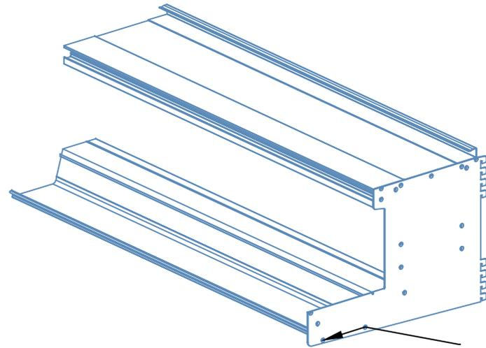
Secure with screws at two positions.
