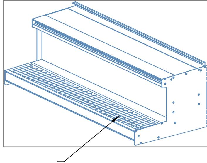
Place the No. 9 leak board on top to complete the installation.
