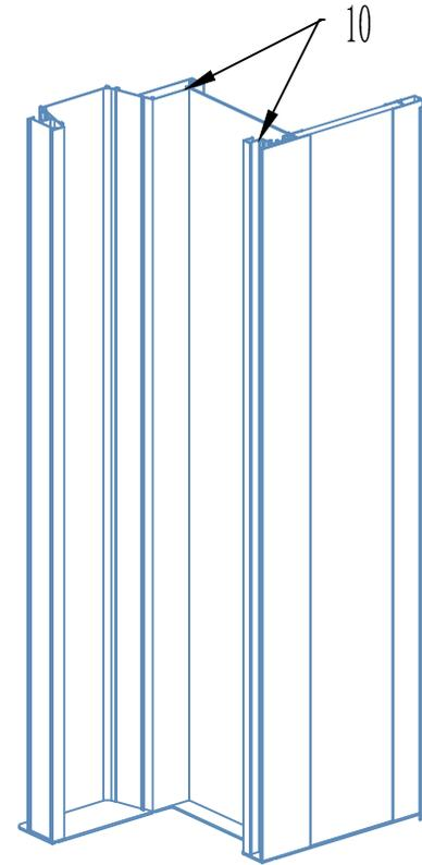
Install the No. 10 panel into the slot between No. 5 and No. 6.
